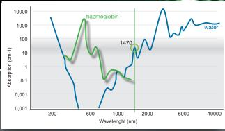
**The Optimal Energy – 1470 nm**The neoV 1470 diode laser offers a novel wavelength with superior performance for ablation of diseased veins – 1470 nm. In contrast to previous generations of laser therapy with deep tissue penetration, the 1470 nm wavelength is highly absorbed by water in tissue. As a result heat generation is highly localized and application is safe and precise.
